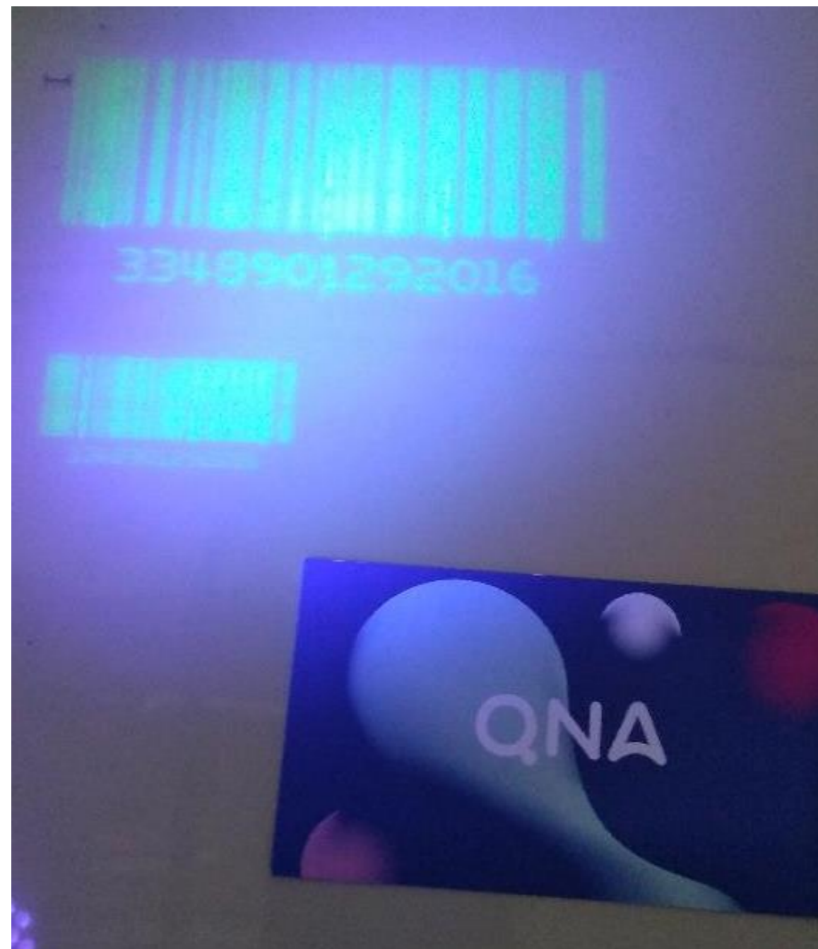
Fluorescent QNA.ink printed on foil with ink-jet office printer.
