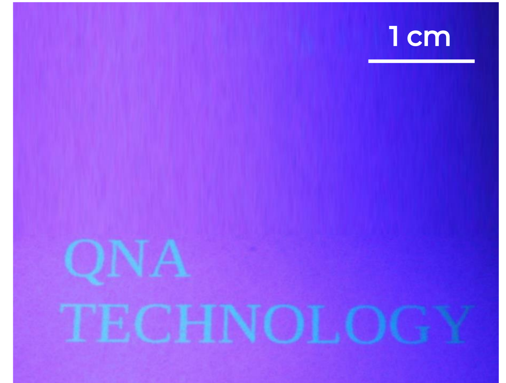
A fluorescent logo printed on paper with QNA.ink with an ink-jet office printer.
