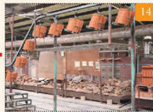
Fired Tile Unloading
