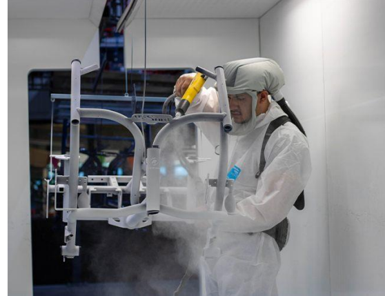
Blasting and power coating
